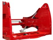
**Hydraulic Stabilizers** – Hydraulic stabilizers are raised and lowered with tractor hydraulics and as an option, a hand pump can be installed for times when a tractor is not available. As well, the gun cart lift is incorporated to raise and lower the cart along with the stabilizers.
